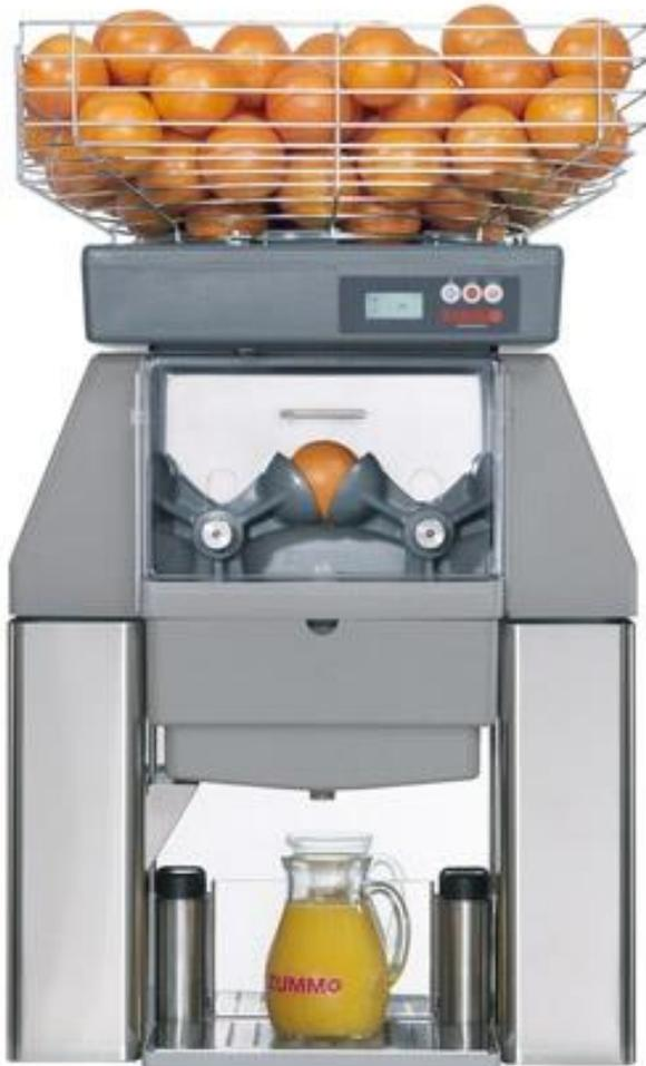
**This is the machine for those businesses that need to produce large quantities of fresh orange/citrus juice. The machine will process 40 fruits per minute (7 to 10kg) producing 2.5 – 3.0 litres per minute dependant of fruit size and yield. That is 1 box of fruit every 2 minutes. 400-600kg of fruit per hour producing 150 – 180 litres per hour.**
